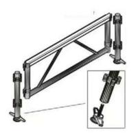
3. Attaching the second braces to the pillar in  $90^{\circ}$  angle, then install the second/third pillar;
