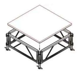
6. Sleeve the adjusting cup and finishing the installation.
